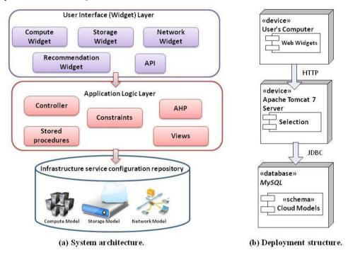
Figure 3: System architecture and deployment structure
