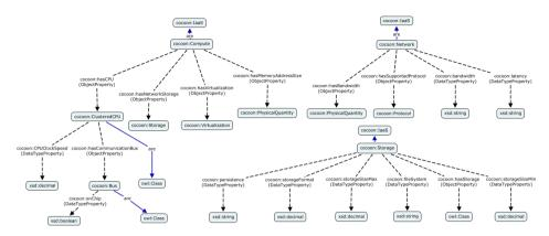
Figure 2: SubClasses and properties for the Compute, Storage and Network class
