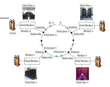
Figure 1. Grid brokers and Grid sites with their Grid peer service and some of the hashings to the Chord ring. Dark dots are the Grid peers that are currently part of Chord based Grid network. Light dots are the publish/subscribe object posted by Grid sites and Grid brokering service.
