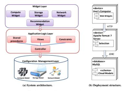
Fig. 1. System architecture and deployment structure
