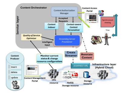
Fig. 8. The MediaWise Cloud architecture [14]
