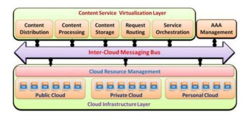
Fig. 9. CoDaaS system architecture
