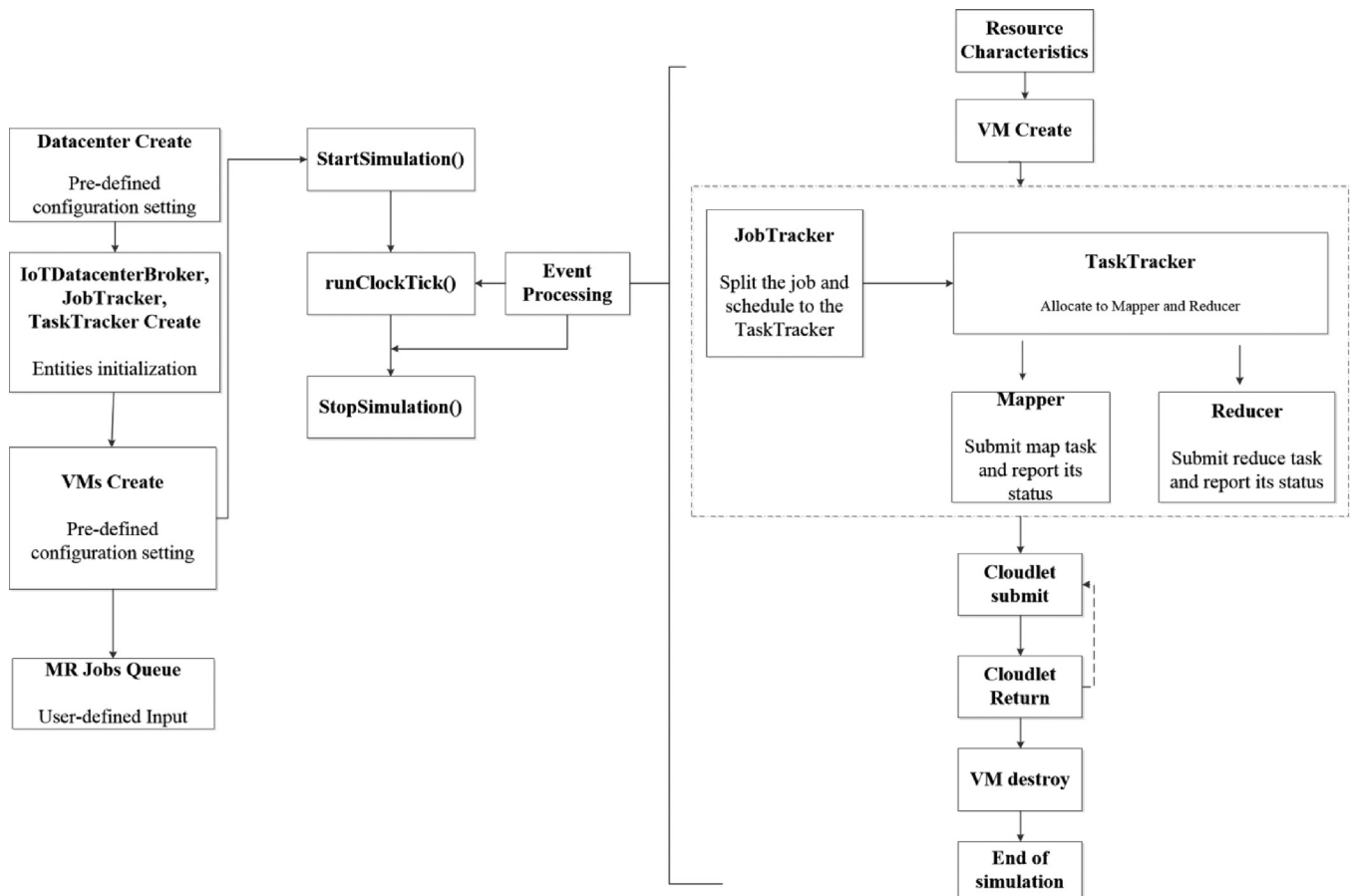
Fig. 7. The basic workflow of how IOTSim works.
