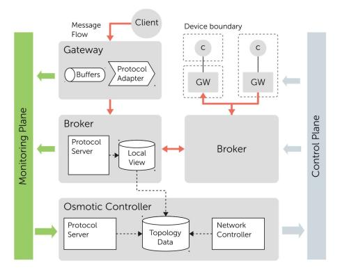
Figure 1. The architectural components of osmotic message-oriented middleware. The osmotic controller orchestrates a network of brokers and gateways via a monitoring and control plane. The gateways transparently connect clients to the system.
