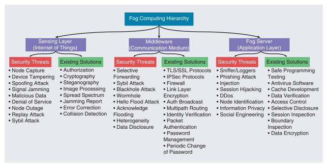
FIGURE 3. The security threats and solutions classifications in fog computing. DDoS: distributed DoS; TLS: transport layer security; SSL: secure sockets layer; IPsec: Internet Protocol security.
