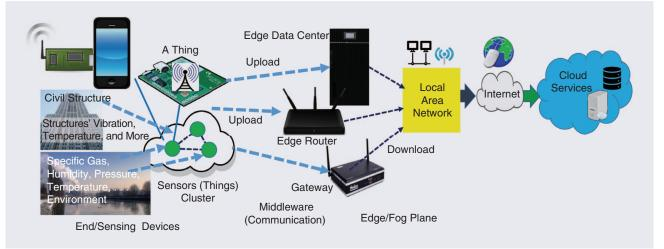
FIGURE 1. The three-layer architecture of fog/edge computing.
