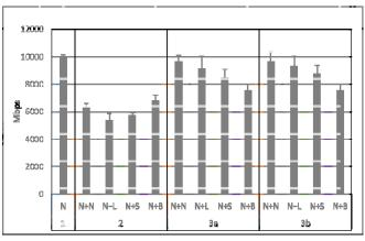
Figure 7. Average Network Performance of Netperf TCP Stream. Black bars on top show the SD.
