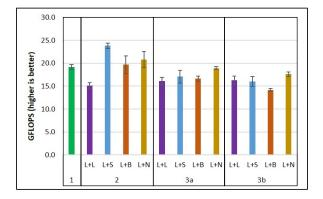
Figure 4. Average CPU Performance of Linpack. Black bars on top show the SD.
