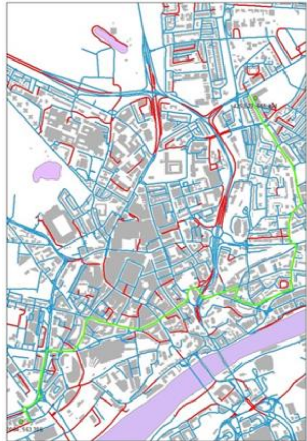
Figure 5. Result of applying a generalised least cost analysis that accounts for disruption to traffic free-flow speeds and flooded roads for part of the city of Newcastle upon Tyne UK.
