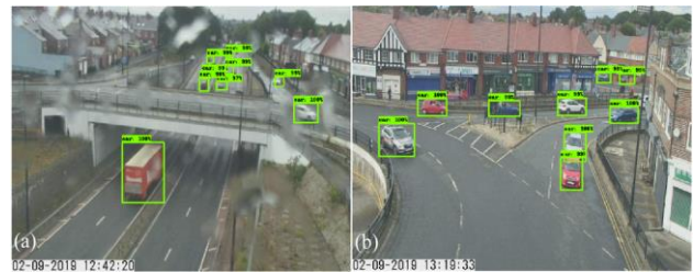
Figure 2. CCTV vehicle recognition using a Convolution Neural Network (R-CNN) for (a) raining conditions, (b) dry conditions.
